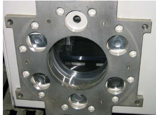
b) Insignificant Deposits on Launch Optics Window
