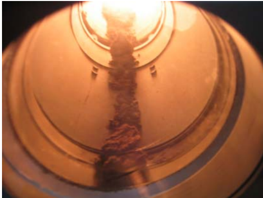
a) Small Amount of Slag Accumulation in Instrumentation Port on Detector Side
