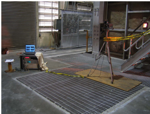
Fig. 2. Detector mounted on a tripod at right, receiving signals from a laser beam passing out of the regenerator section of a float glass furnace. The LTS-100 processing unit can be seen on the left.
