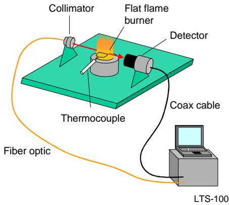
**Figure 4. Experimental setup for calibration of the LTS-100 with a thermocouple in a premixed flat flame.**
