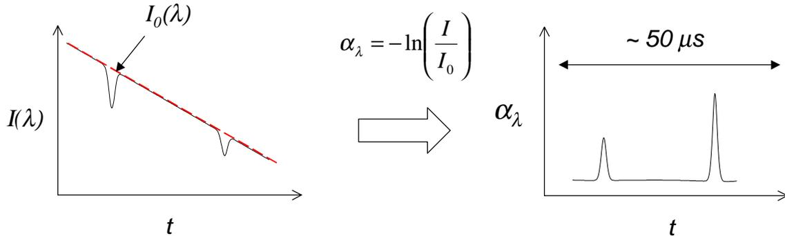
**Figure 3. Scanned wavelength technique for measuring spectral absorbance.**
