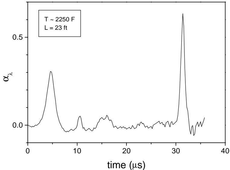
**Figure 8. A typical H<sub>2</sub>O absorption scan measured *in situ* at the TVA Kingston plant over a 23-ft path.**
