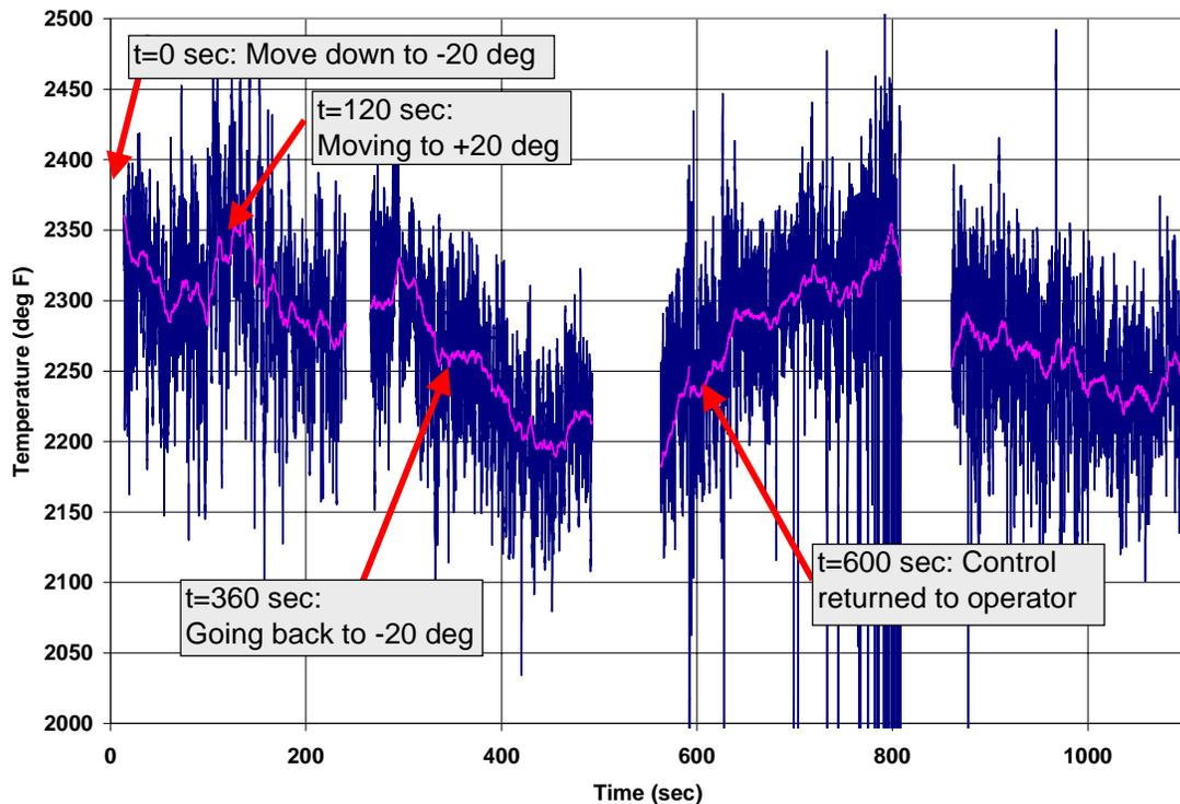
**Figure 9. Time history of temperature from the line area ratio from *in situ* measurements at the TVA Kingston coal fired power plant during various positions of the burner tilt angle.**
