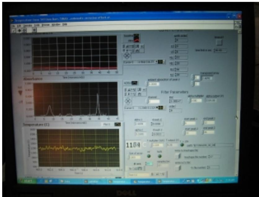
**Figure 7. Screen shot of the LTS100 software during operation at the TVA Kingston coal-fired powerplant.**
