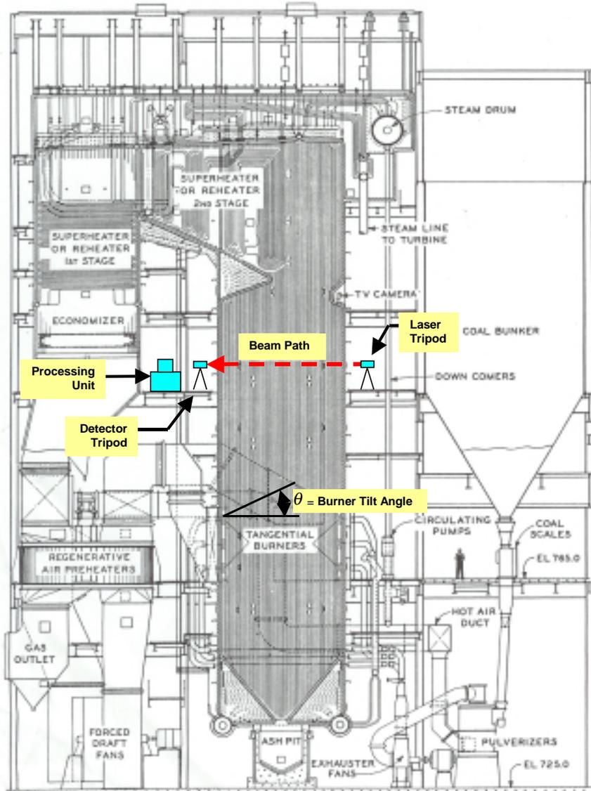
**Figure 6. Side view of the experimental setup during in situ temperature measurements on Unit 9 of the TVA Kingston plant.<sup>12</sup>**
