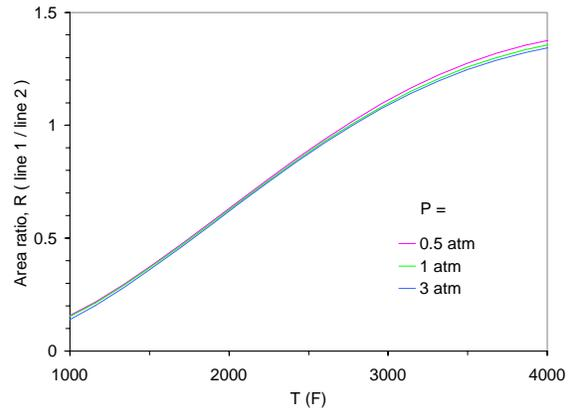
**Figure 2. Simulated area ratio of H<sub>2</sub>O line pair near 1500 nm.**
