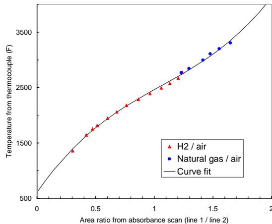
**Figure 5. Experimentally obtained calibration curve for the LTS-100 system.**
