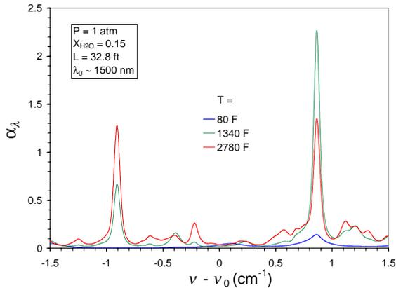
**Figure 1. Simulated H<sub>2</sub>O absorbance spectrum near 1500 nm showing two features that have different temperature dependence.**
